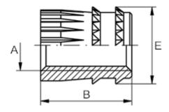
Female thread A = M2 Length B = 4.0Max outer diameter E = 4.0Number of cramping feathers = 1
